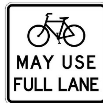
MUTCD sign for narrow travel lanes that require sharing
